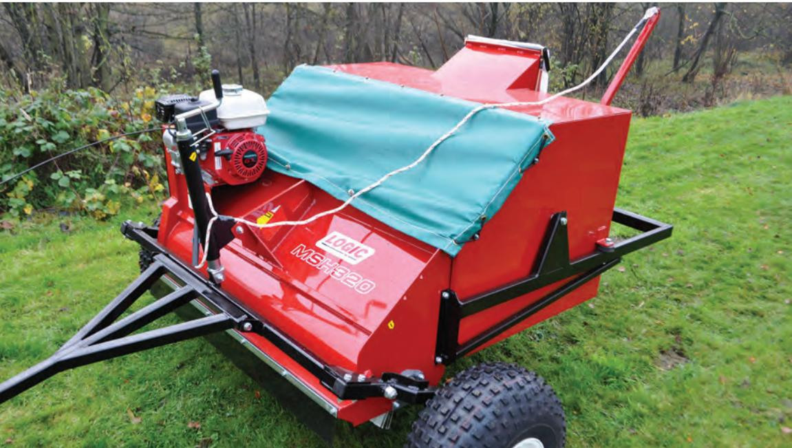
The MSH320 has a 1.2 metre working width with large 22x11-8 flotation front tyres and 18x8.5-8 castor rear tyre for use on soft ground/rough conditions. It has a manual height adjustment screw to provide a range from 75mm to 300mm.
