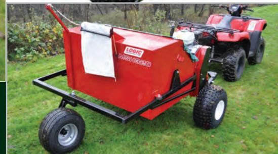
This model features a 600 litre capacity hopper with tipping rope and single pivot point. The contents would typically be tipped onto a tarpaulin or sheet for further processing before drying and cleaning (as shown right).
