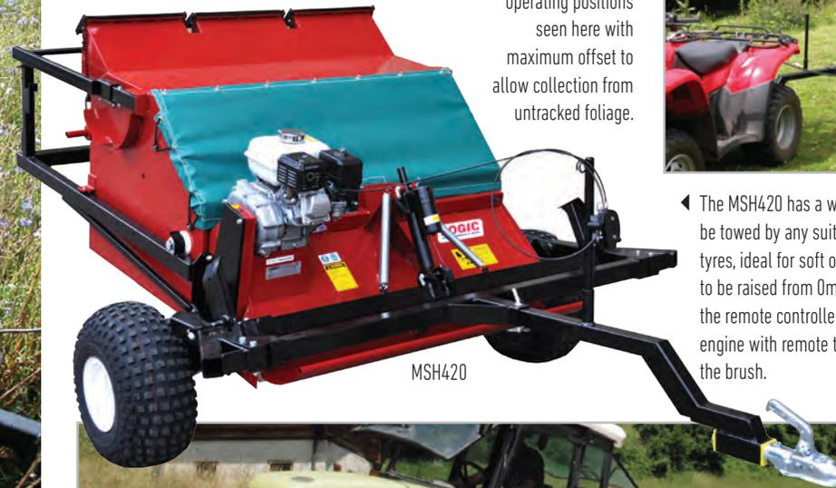
◀ The MSH420 has a working width of 1.2 metres and can be towed by any suitable vehicle. Large 22 x 11-8 flotation tyres, ideal for soft or rough conditions, allow the brush to be raised from 0mm to a maximum of 525mm, using the remote controlled electric actuator. A 5.5hp Honda engine with remote throttle and centrifugal clutch drives the brush.
