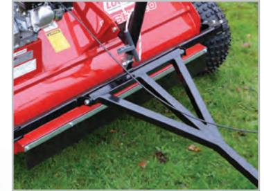
This model has a simplified drawbar and is towed in the central position.
