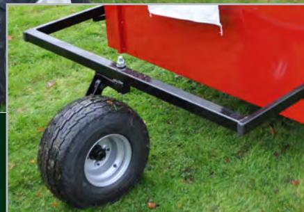
Flotation wheels, including this rear castor wheel, are fitted as standard to ensure easy towing by any suitable vehicle over soft or rough ground conditions.
