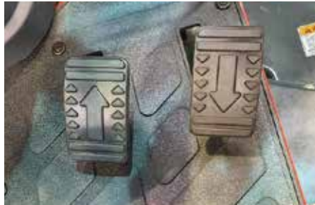
2. Dual hydrostatic control pedals for smooth forward and reverse transition.
