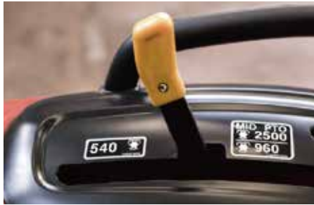
2. Easy to use PTO is standard with rear 2 speed and mid 1 speed.
