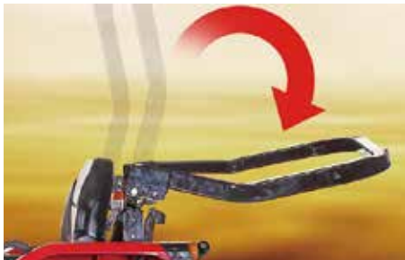
4. Foldable ROPS enables low clearance operation, ideal for working under trees.
