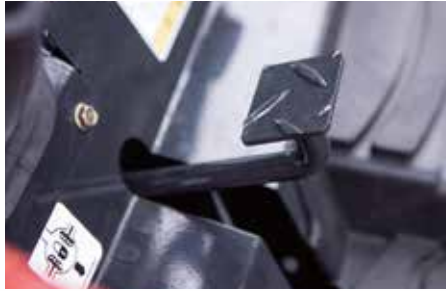
2. Differential lock system improves traction on slippery surfaces with an easily accessible foot pedal.
