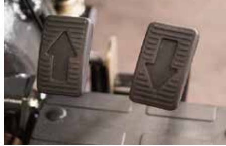
2. Dual hydrostatic control pedals for smooth forward/reverse (only for HST model).
