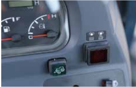
1. Simple one touch button to engage electronic cruise control.
