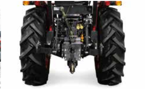
6. The category I hitch has a lift capacity of 1,500kg at the ball end and 1,000kg measured 610mm rearwards behind the balls.
