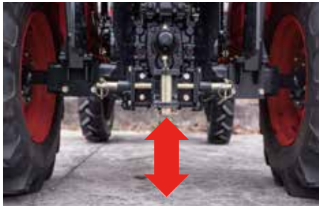
4. High ground clearance is excellent for protecting crops.
