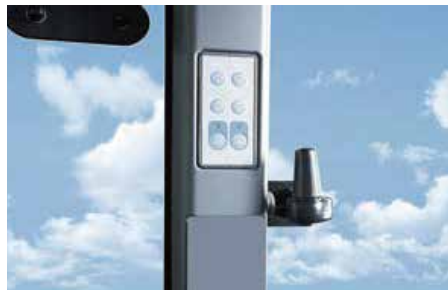
5. Easy access to the button-panel light controls located on the inner pillar of the cab.
