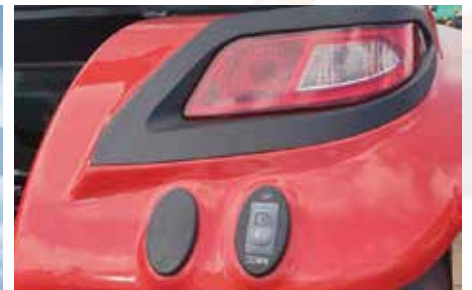
6. Exterior three point linkage lift arm control switch located on the rear fender for easy fine control while attaching implements
