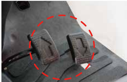
5. Dual hydrostatic control pedals for smooth forward/reverse (only for HST model)
