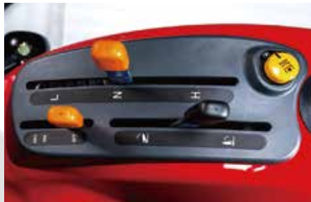
5. Easy control of PTO operation and selective 4WD depending on applications.
