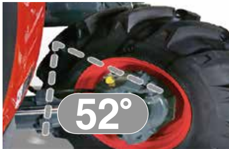
5. 52° turning angle makes it easy to operate in narrow areas.
