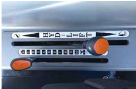
2. Three point linkage and draft controls for precise raising and lowering of implements.
