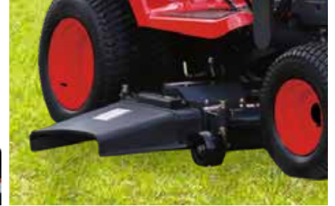
3. Quick and easy installation of 54inch (1.5m) mid-mounted mower available.
