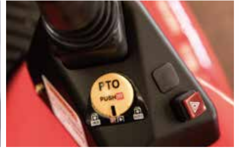
3. PTO operation - optional electro-hydraulic: a) Fully independent b) Linked to adjustable height of 3PL
