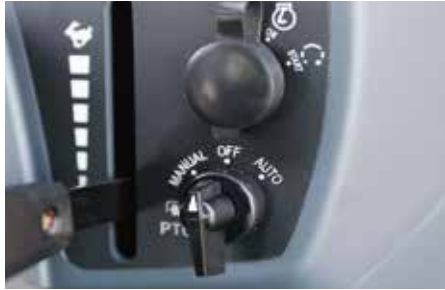
2. PTO operation - optional electro-hydraulic: a) Fully independent b) Linked to adjustable height of 3PL.
