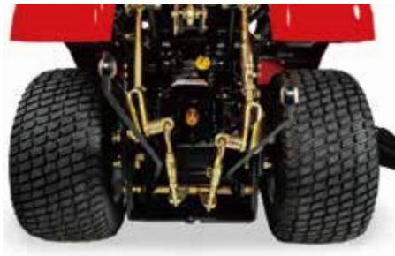
4. Category I 3-point hitch with 499kg lift capacity.
