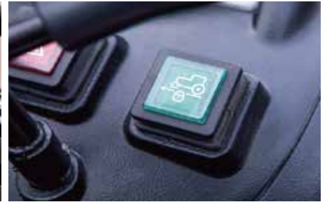
3. Simple one touch button to engage electronic cruise control.
