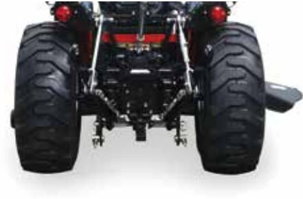
1. Category I with a hitch-lift capacity of 600 kg allows for usage with a wide variety of implements.
