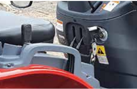
4. Mechanical cruise control lever to maintain constant forward speed during mowing or seeding tasks.
