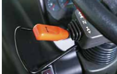
2. Power shuttle lever enables easy forward and reverse shifting.
